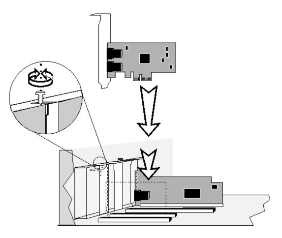
Figure 1. Insertion of the adapter into the computer
